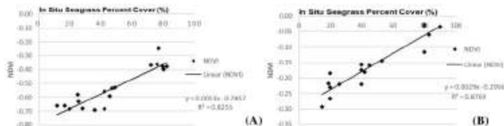
Fig. 9 Correlation analysis of SPC between in situ measurement and NDVI values on the three islands: A Sentinel-2 imagery, B Landsat 8 imagery
